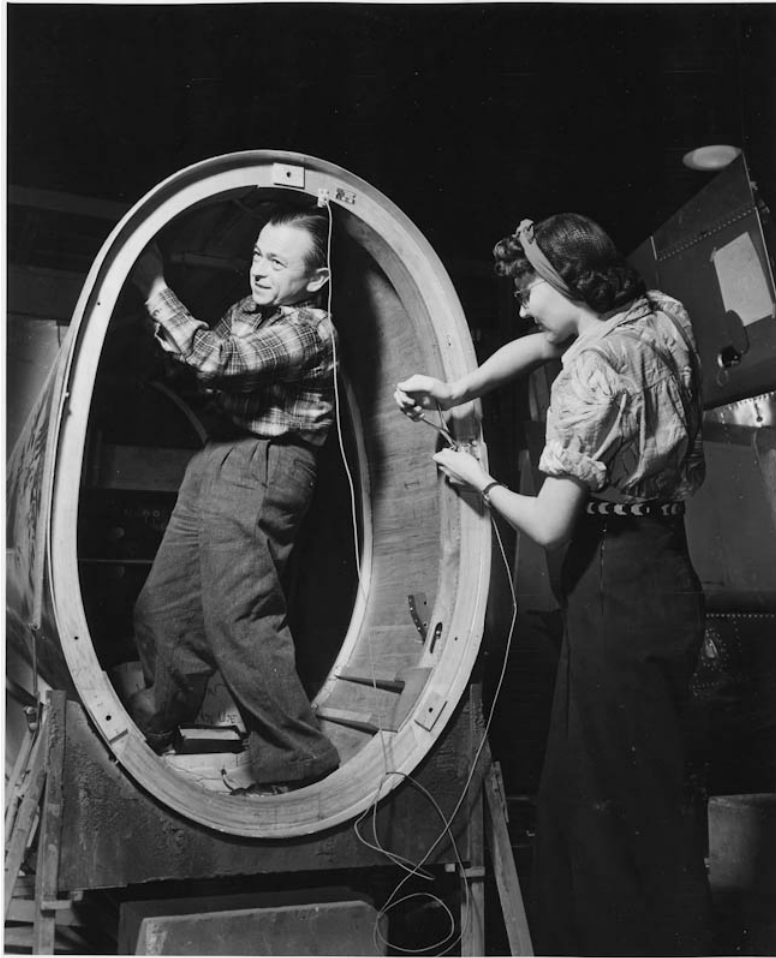
Figure 5.3: “A [Little Person] and a woman worker install control wires on a “Valiant” basic trainer. At the Downey plant is made the BT-13A (“Valiant”) basic trainer - a fast sturdy ship powered by a Pratt & Whitney engine.” Courtesy of Franklin D. Roosevelt Library.
