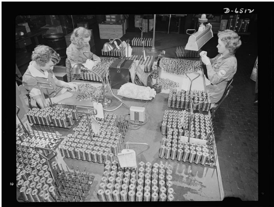
Figure 4: Pratt and Whitney workers inspect tappet rollers for airplane engines in June 1942 (Credit: Library of Congress)
