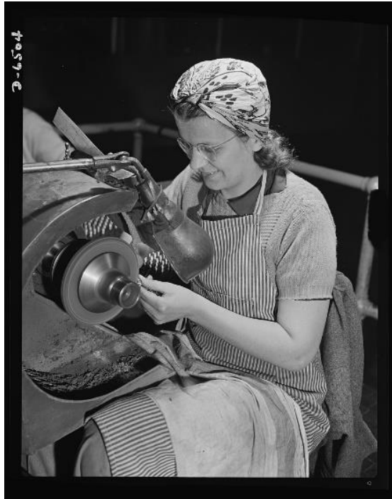
Figure 3: A Pratt and Whitney worker polishes screws for valve rocker arms for airplane engines in June 1942 (Credit: Library of Congress)
