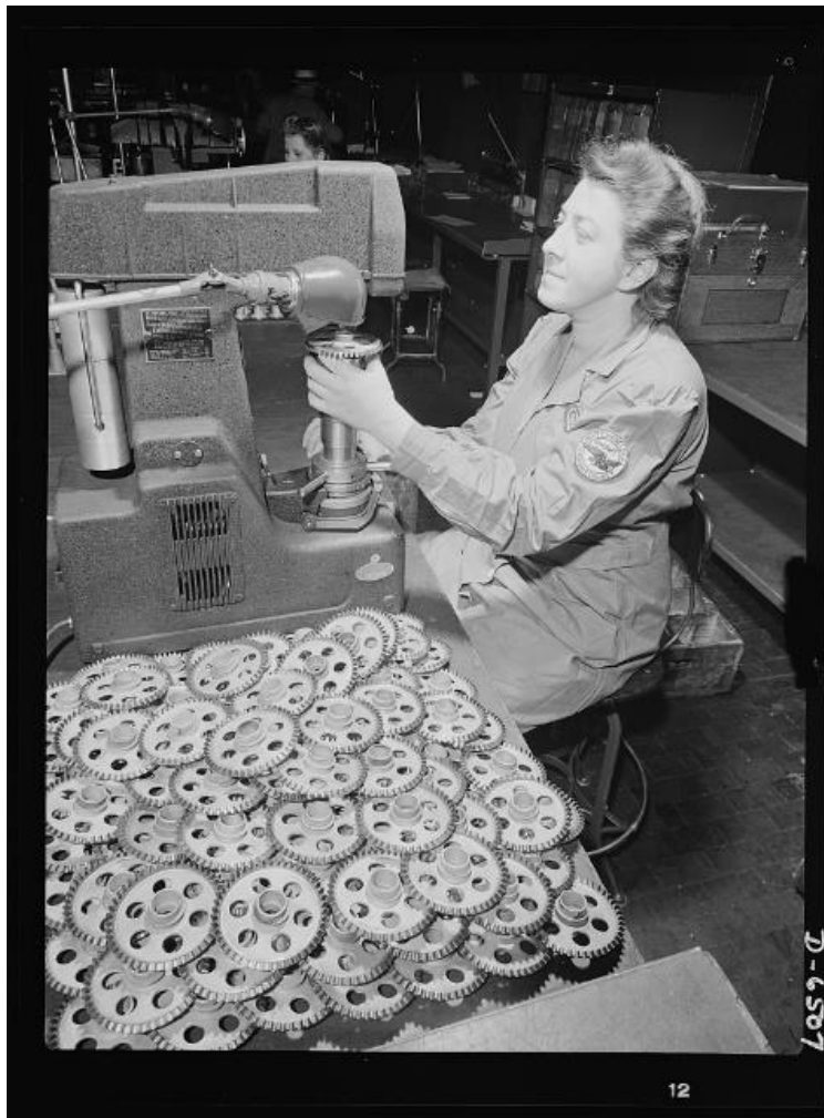
Figure 2: A Pratt and Whitney worker tests magneto driving gears for hardness on a Rockwell machine in June 1942. (Credit: Library of Congress)
