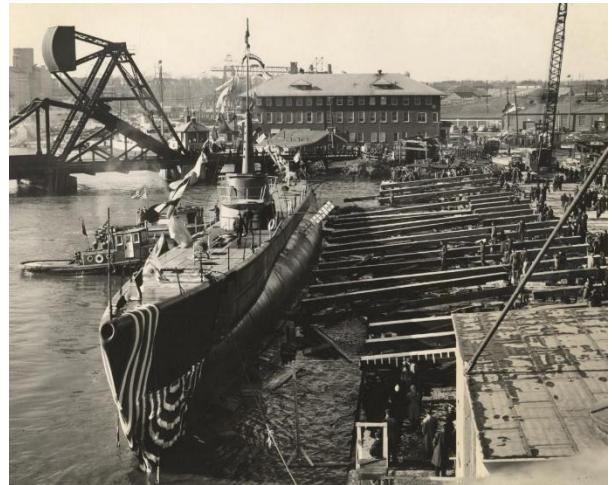
The submarine USS Hardhead on December 12, 1943, just after launching at the Manitowoc Shipbuilding Company. Credit: P92-5-86, Wisconsin Maritime Museum Collection, copy and reuse restrictions apply.
