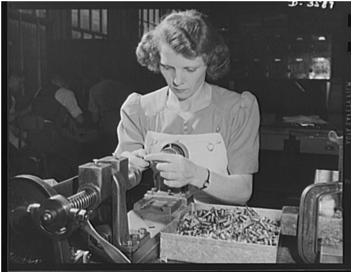
Figure 21: “Conversion. Cash registers to gun magazines. A boring operation on the Oerliken machine for 20mm anti-aircraft guns. Many regular employees were retained when a large cash register manufacturing plant changed over to war production. National Cash Register Company, Dayton, Ohio,” February 1942 (Credit: Library of Congress)
