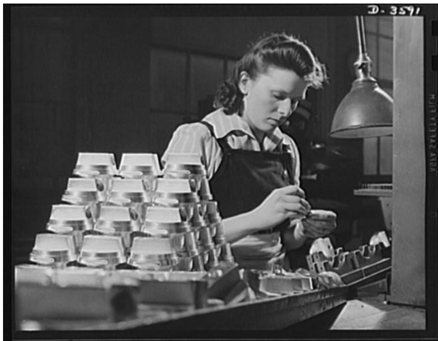
Figure 9: "Conversion. Cash registers to gun magazines. Assembly of M-48 fuse bodies. Huge quantities of these war essentials are coming off the production line of a converted cash register plant. National Cash Register Company, Dayton, Ohio," February 1942 (Credit: Library of Congress)
