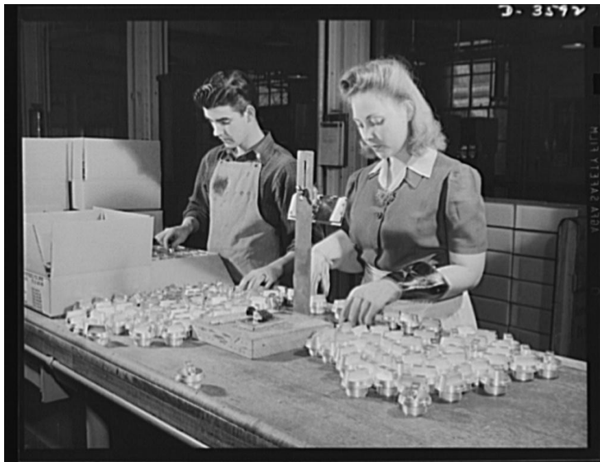
Figure 8: "Cash registers to gun magazines. Women work side by side with men to smash the Axis. Arming test of M-48 fuse bodies part of the routine inspection of shell parts at a former cash register factory now engaged in war production. National Cash Register Company, Dayton, Ohio," (February 1942) (Credit: Library of Congress)
