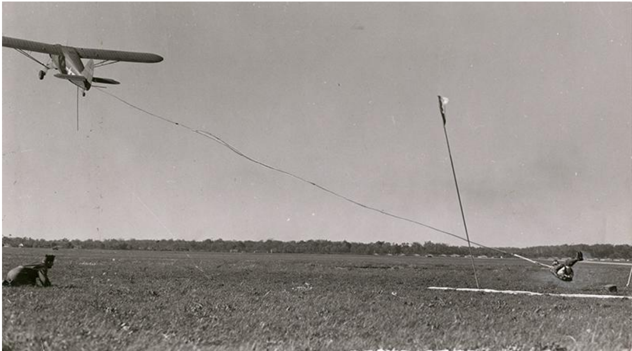
Figure 11: Experimenting with picking up a man on the ground by a flying aircraft, 1943, Wright Field. The plane is a Canadian-built UC-47 Norseman. (Credit: Wright State University Archives)
