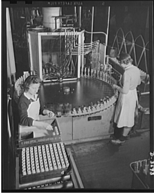
Figure 10: “Cash registers to gun magazines. A machine (with women workers) paints the exterior and interior of each 37mm M-54 high explosive shell made at a former cash register factory now engaged in war production. National Cash Register Company, Dayton, Ohio, ” February 1942 (Credit: Library of Congress)
