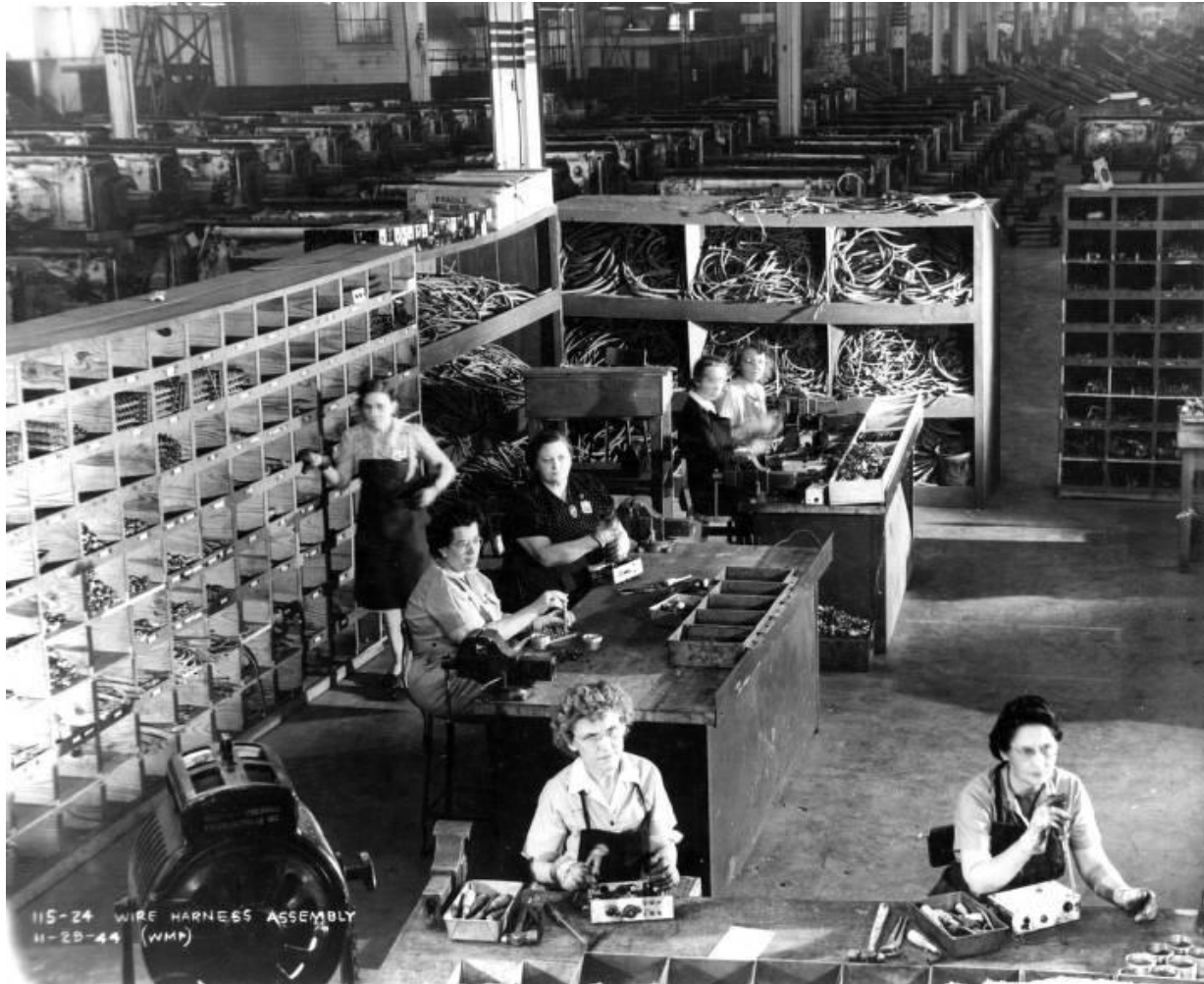
Figure 6: Wire harness assembly at the Evansville Ordnance Plant at the Chrysler plant in Evansville, Indiana, November 29, 1944 (Credit: University of Southern Indiana, Rice Library Digital Collections)
