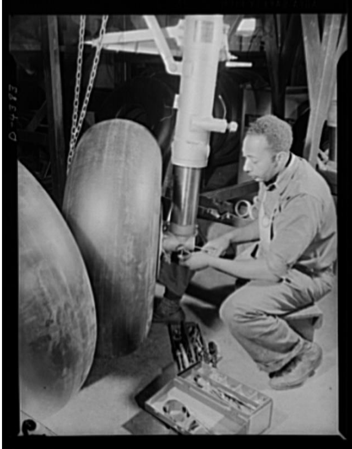
Figure 7: This worker is assembling landing gear for a medium bomber and learned his craft under the government war training program. Pictured at Glenn L. Martin Bomber Plant. May 19, 1942. (Credit: John Collier Jr., Library of Congress)
