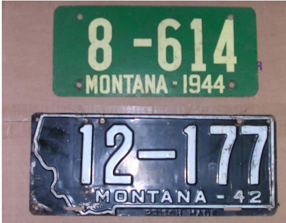
Figure 14: 1942 Montana license plate (bottom of photo), made of tin. 1944 Montana plate (top of photo) is made of soy meal. (Courtesy of Gary Yaeger)
