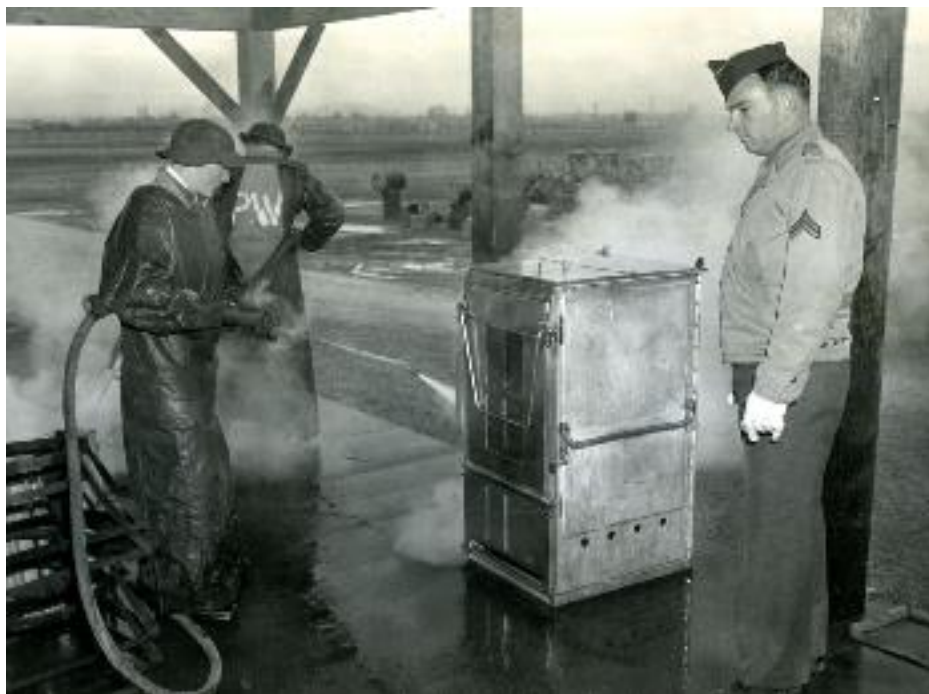
Figure 21: German POWs at work at Defense Depot Ogden under the supervision of a Corporal. They are cleaning field ranges with steam. Their clothing is marked with "PW" for identification. Photo by the U.S. Army Signal Corps. (Credit: Special Collections Department, Stewart Library, Weber State University, ID 99153)
