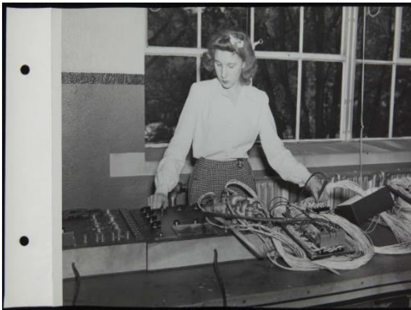
Figure 23: Woman Making Electric Harnesses for B-24 Bombers at the Phoenix Mill (Credit: From the Collections of The Henry Ford.)
