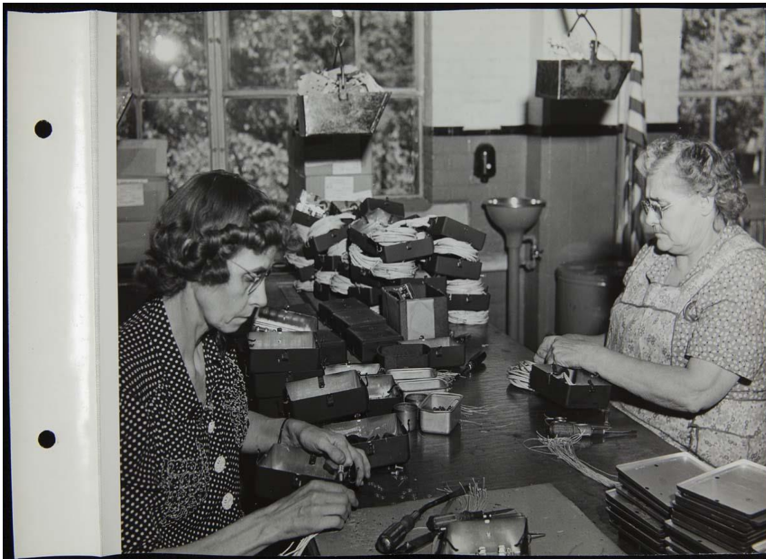
Figure 3: Women Making Electric Harnesses for B-24 Bombers at the Phoenix Mill (Credit: From the Collections of The Henry Ford.)
