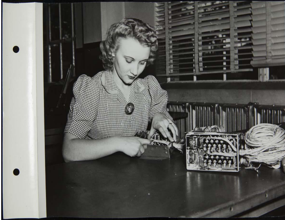
Figure 6: Woman Making Electric Harnesses for B-24 Bombers at the Phoenix Mill (Credit: From the Collections of The Henry Ford.)
