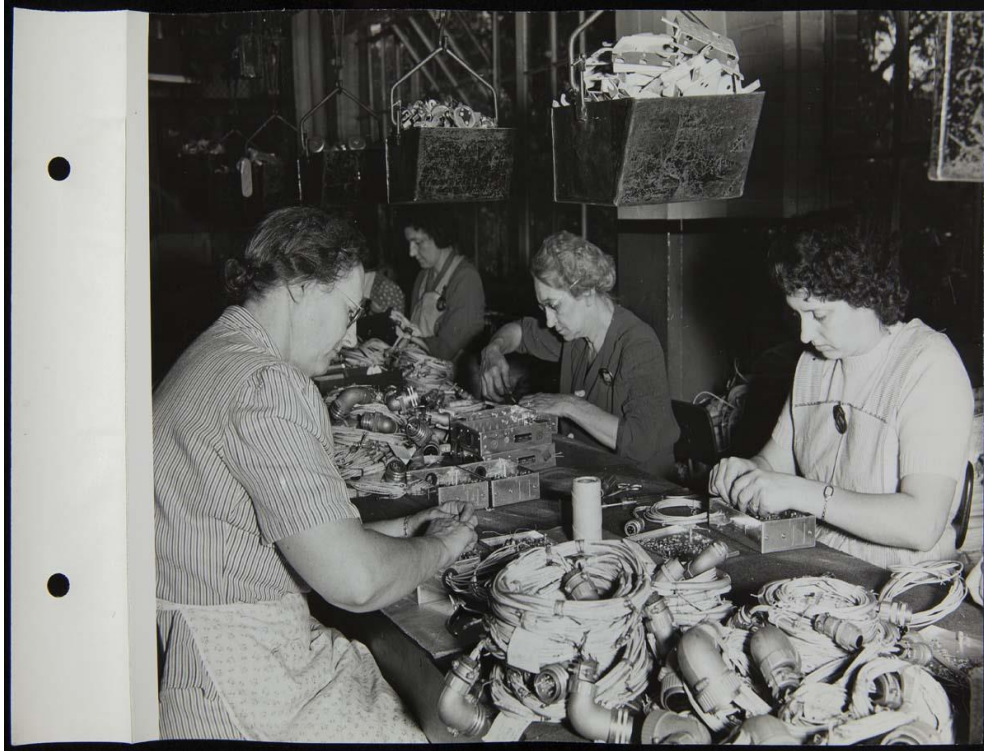
Figure 4: Women Making Electric Harnesses for B-24 Bombers at the Phoenix Mill (Credit: From the Collections of The Henry Ford.)
