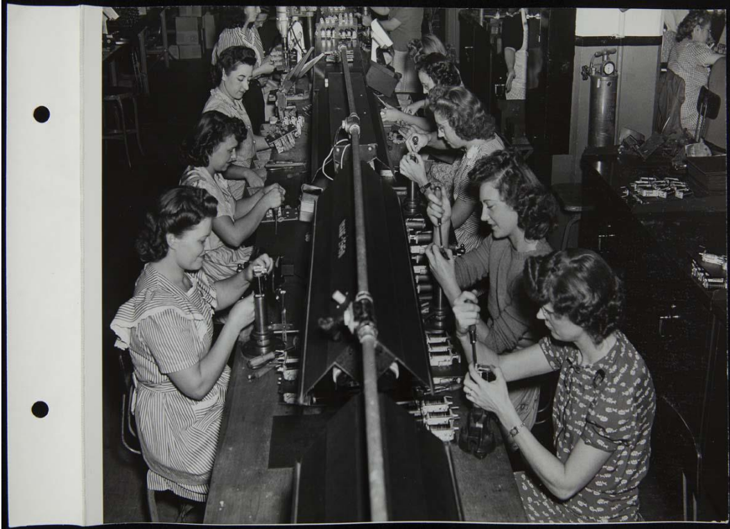
Figure 1: Women Making Electric Harnesses for B-24 Bombers at the Phoenix Mill in Plymouth Township, Michigan. (Credit: From the Collections of The Henry Ford.)
