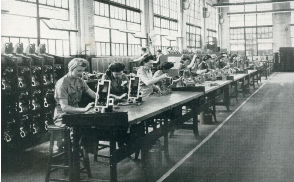
Figure 16: Women workers inspect Lawrance crank cases for Army specifications at Otis Harrison Works. (From “War Production” by Otis Elevator Company (1947), Credit: Yonkers Public Library)
